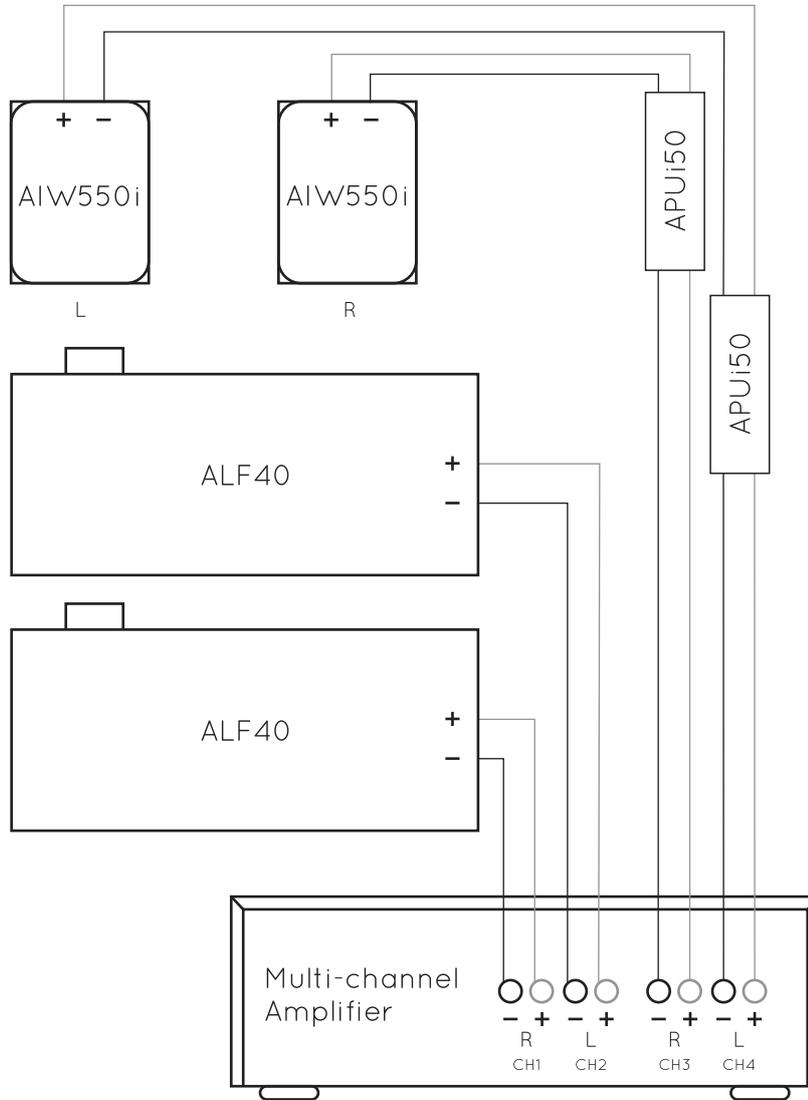
For systems using a pair of AIW550i speakers, two ALF40's will be necessary. In this scenario the amplifier will need four independent channels.
