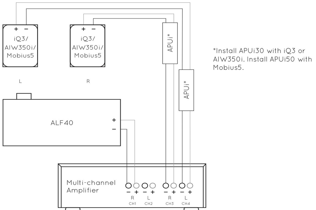
By connecting a single ALF40 to its own amplifier channel, its output (relative to the iQ3/ Mobius5/ AIW350i pair) can be set optimally. In larger rooms care should be taken not to adjust the relative output of the ALF40 too high. This may result in the unit reaching its mechanical limits well before that of the accompanying Amina speakers. If this is the case, consider using two ALF40's (Active Stereo 2. 2) or an ALF80 or ALF120.
